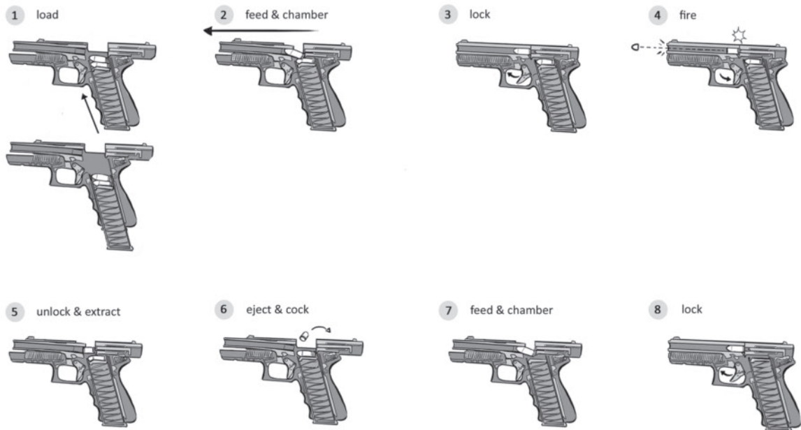
Figure 3-4 Cycle of operation for a semiautomatic pistol
