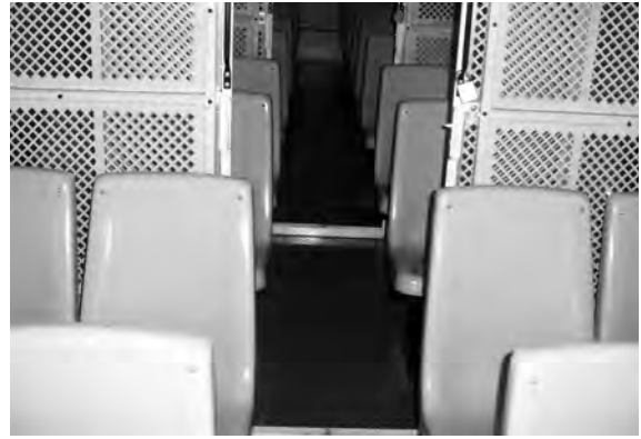
Figure 6-2: Example of a typical transport vehicle with partitions and screens
